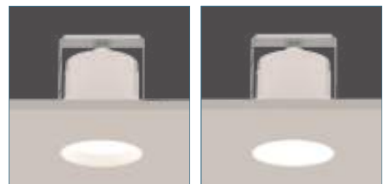
RECESSED POSITION FLUSH-FITTED POSITION
