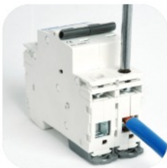
Safety terminal: easy wiring; protection degree IP20. Positive and slot screw head. Torque up to 2,8 N·m.
