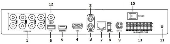
\*: This corresponds to the rear panel of TBK-DVR1208. The rear panel of TBK-DVR1204/1216 provides 4/16 video input interfaces, 4 alarm in, and 1 alarm out.
